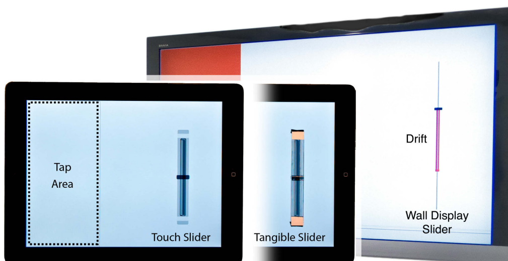
Figure 6.17: The tablets with the unembodied touch control (left) and the embodied tangible control (right) in front of the wall display showing also a slider and the participant's drift relative to a pre-computed 1D path.
