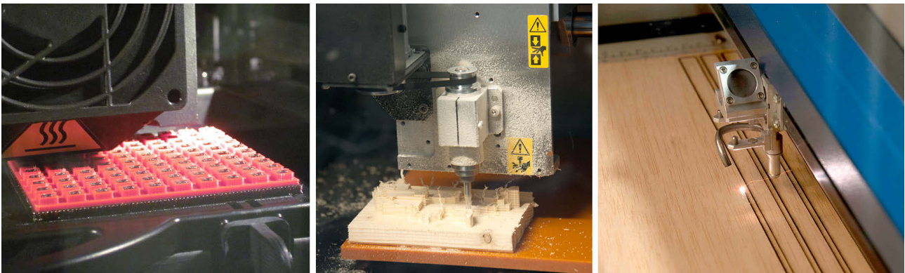
Figure 7.1: Common machines for digital fabrication: 3D printer, 3D milling machine, 2D lasercutter.
